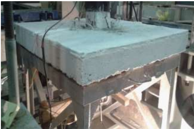
Figure 8: The loading test setup
