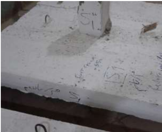
b) Slab S1 - Compression side
