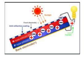
Figure 7: Photovoltaic Effect, [31]
