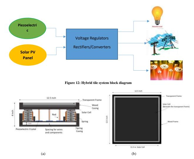
Figure 13: Hybrid PV-Piezo floor tile (a) cross section view of internal components (b) top view of the hybrid tile[32]
