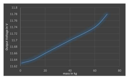
Figure 6: Varying the output voltage of piezoelectric transducer for different weights
