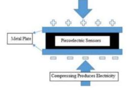
Figure 2: Piezoelectric mechanism and effect[18]
