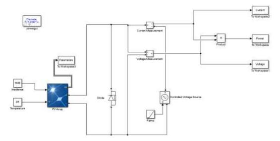
Figure 9: PV array simulation model
