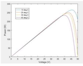
Figure 10: V-P curve of the simulated PV array
