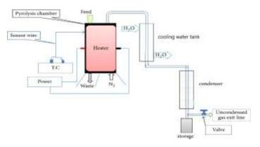
Figure 2 pyrolysis process
