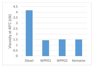
Figure 7 viscosity comparison
