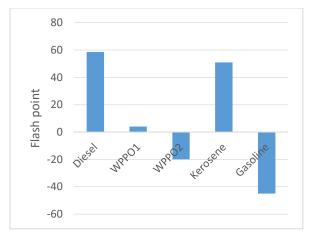
Figure 9 flash point comparison
