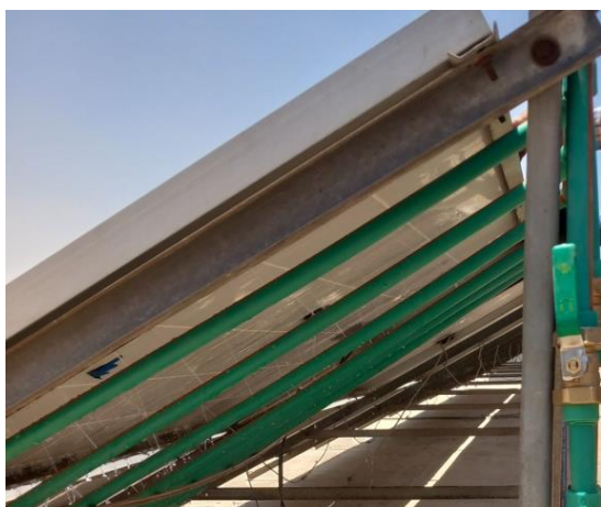
Fig. 1: Water back cooling system for PV panel
