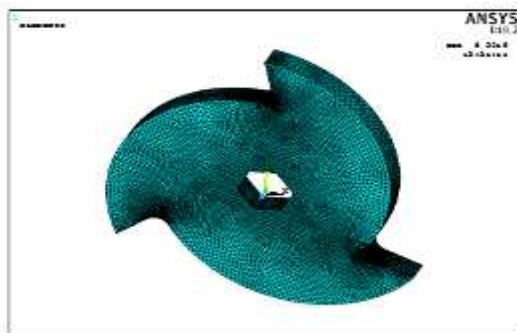
Figure 5: Shredder Blade Meshing
