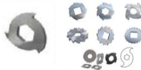
Figure 2: Types of shredder blades
