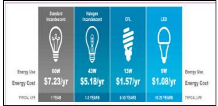
Figure 2: Common Bulb Technologies with Annual Electricity Cost, [15]
