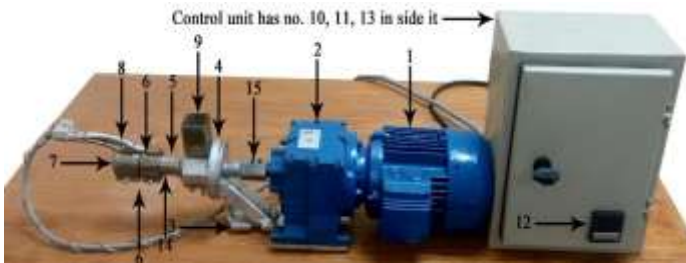
1 Motor 2 Gear box 3 Base A 4 Base B 5 Housing 6 Heaters 7 Screw 8 Temp. sensor 9 Hopper 10 Inverter 11 direction switch 12 Thermostat 13 Relay 14 Oil collector 15 Coupling
